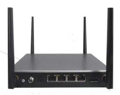
The NCA-1040, a fanless multi-service gateway with Intel® Atom X6413E CPUs, addresses the growing need for Edge security and CPE due to the widespread use of mobile devices and their diverse applications.
