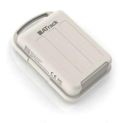
AS300 rechargeable device ensures versatile applications and cost savings. Enjoy extended battery life – 2 weeks at 60-minute intervals or 2 days at 1-minute intervals. Waterproof and durable, ideal for outdoor use. Connect and monitor multiple devices simultaneously with BLE sensors for efficient tracking.
