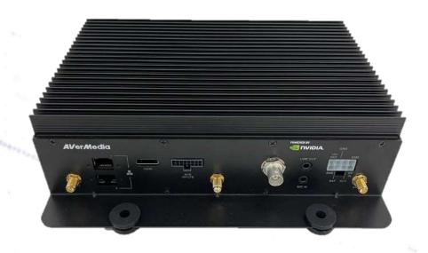
The AVerMedia AI Box PC built with NVIDIA Jetson Nano module is tailored for fleet management and smart security, supporting four AHD 1080p 30 image analyses concurrently. It offers superior stability and inference performance over Intel X86 systems.
