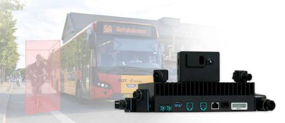
oToGuard is equipped with 1 automotive-grade ECU system, 8 cameras, and vision-AI deep learning technology to realize multiple ADAS functions in order to protect vulnerable road users 360 degrees and monitor driver's behaviors to prevent accidents from happening.
