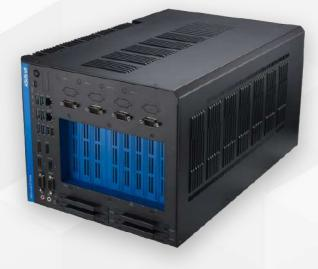
Rugged edge AI GPU computer supporting up to dual 450W GPU cards for AI computation
