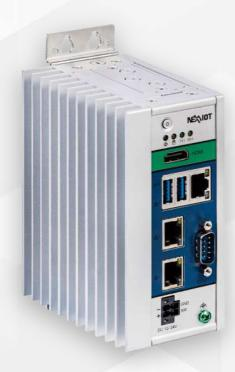
The NIFE 106 Factory Automation Fanless System, featuring a palm-sized form factor, is powered by the Intel® Processor N97 Quad-Core.
