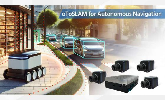
oToSLAM utilizes vision-AI technology, 4 automotive cameras, and an ECU to enable multi-camera vision-AI SLAM system.
