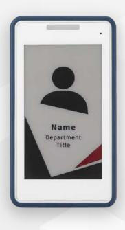
A 3.7-inch NFC-powered, battery-free ePaper display, designed for an ultra-slim form factor and enabling quick image updates via mobile devices and NFC readers. The EPD-303 supports black, white and red colors for versatile display options.
