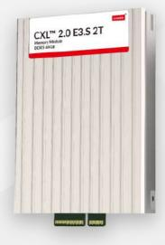
Capacity: 64GB Interface: By PCIe 5.0 / E3.S 2T Supported Platform:
