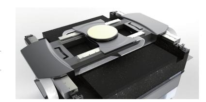
The precision positioning stage is an essential machine for manufacturing semiconductors. If silicon, the semiconductor material, is placed on the disk (stage), the disk moves vertically and horizontally with nano-meter-level motions according to the computer program. In response to the motion, electronic ponents and circuits are printed from above.
